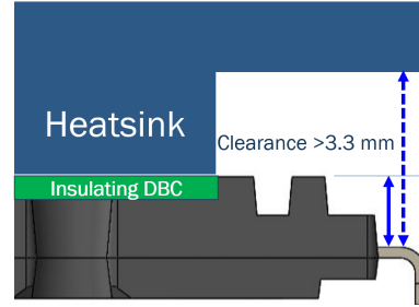
Figure 17. Illustration of Achievable Clearance
