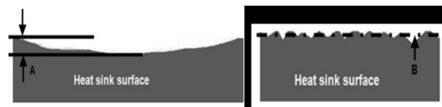
Figure 19. Flatness (a) and Roughness (b) of the Heatsink
